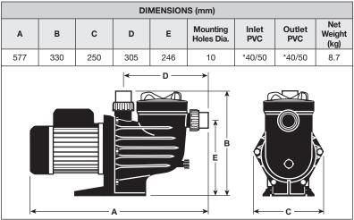
Suction & delivery accept 40mm PVC pipe on the I.D. and 50mm fitting on the O.D.
