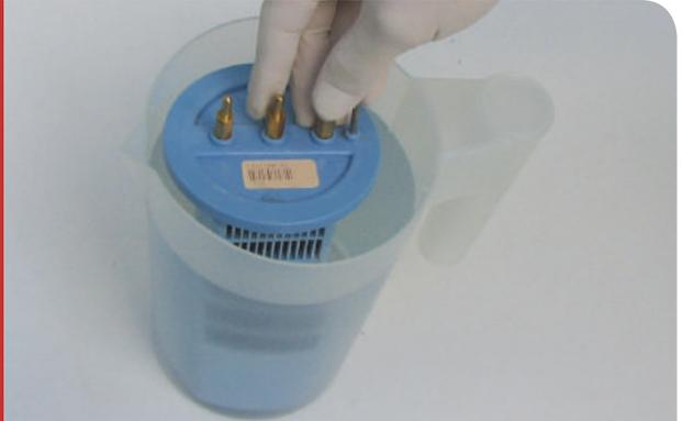
There will be a reaction as the calcium is dissolved. When the reaction ceases (about 10 minutes) rinse the electrode in clean water, wipe the brass terminals dry and check that all calcium has been dissolved. If not, repeat the process with a new solution.
