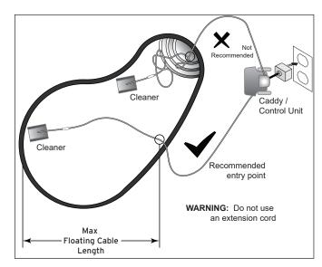
Figure 15. Optimal Entry Point in Pool
