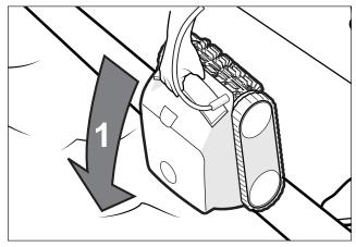
Figure 11. Submerge the Cleaner Vertically
