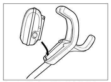
Figure 8. Align Control Unit with Caddy Hook
