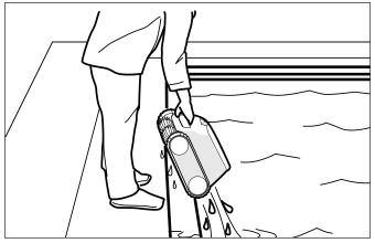
Figure 16. Keep Cleaner Vertical to Drain Water
