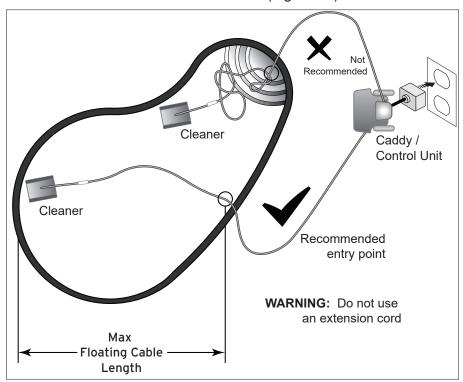
Figure 13. Pool Entry Point for Optimal Patterning
