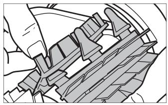
Figure 29. Pull Tabs Through Each Slot
