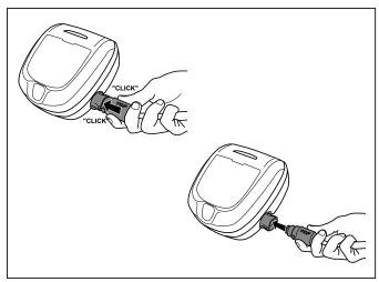
Figure 10. Remove Protective Cap and Connect Power Cable
