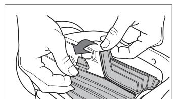
Figure 27. Undo the Tabs of the Brush
