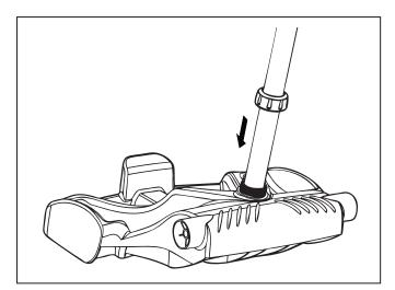
Figure 4. Twist Handnut to Secure Frame
