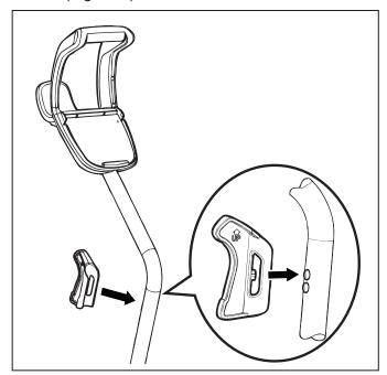
Figure 7. Snap Cleaner Hook into Place
