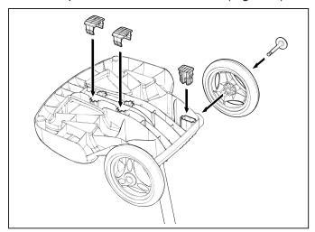
Figure 5. Snap in Support Blocks and Attach Wheels
