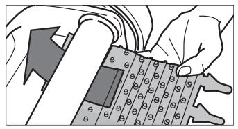
Figure 28. Position the New Brush on Roller
