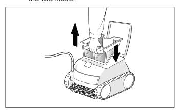
Figure 21. Separate Filter Canisters
