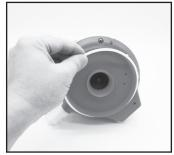
2. Use the screwdriver to unscrew the 4 screws located at the bottom of the head to release the bottom plate first. Then unscrew all the screws at the base as shown. Remove the impeller and pry open the base to expose head inside.
