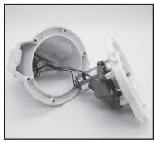
3. Remove out the battery pack to expose the PCBA. To detach the battery connection wire, press on the clip of the connector to pull it out. **NOTE:** Wrap the connector immediately with insulating tape in order to avoid any short circuit caused by the contact of both wire terminals.
